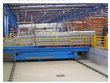
The system had to be flexible enough to work with trucks of various tray heights and lengths as well as with shipping containers of up to 40 feet length.
