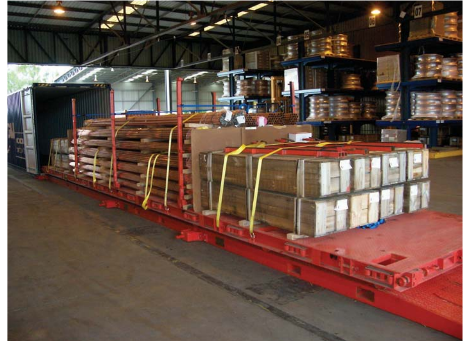
A 40 ft SLC offers the flexible loading for both long and short pieces.
