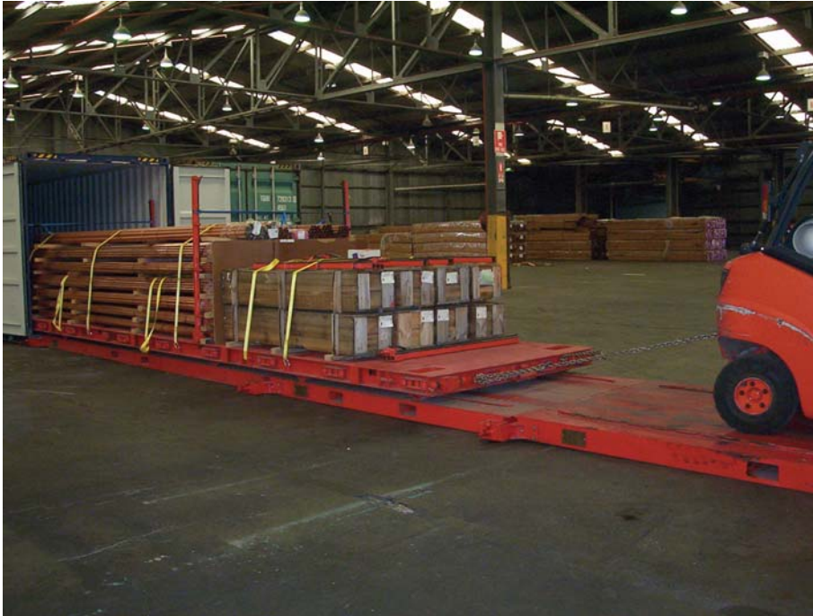
A load of Copper towed out on a 40 ft SLC with side supports.
